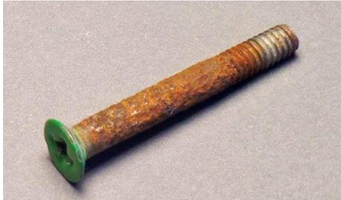
Figure 18: Steel bolt after 30 years in wood longeron
