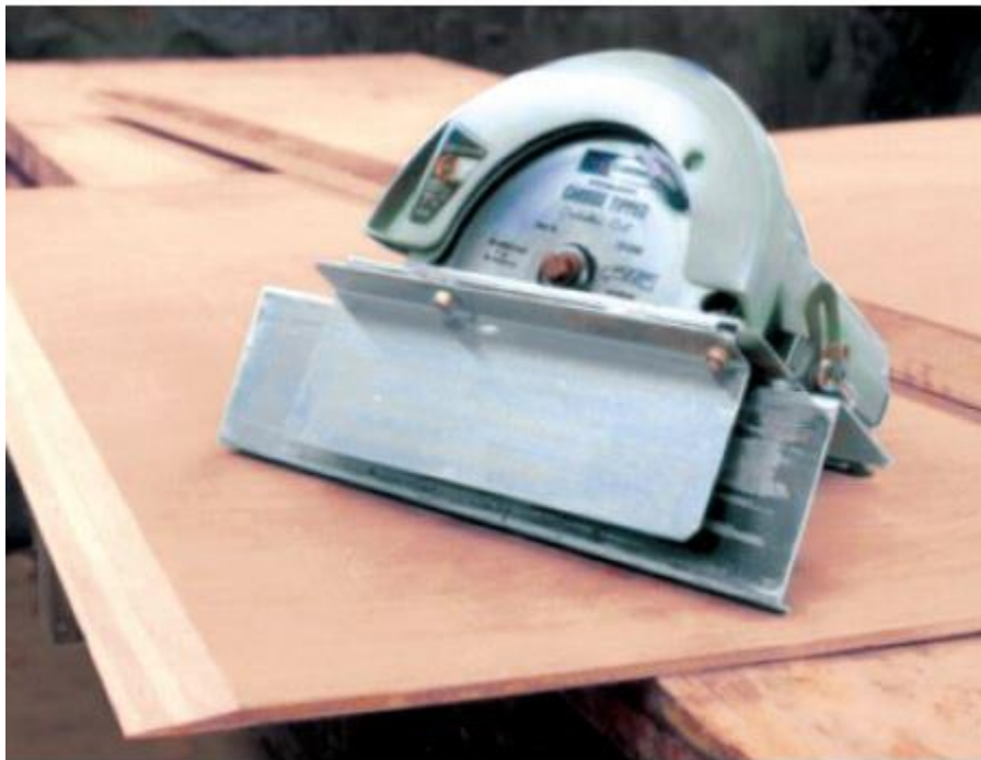
Figure 8: Commercial Scarfing Attachment for a Circular Saw.
