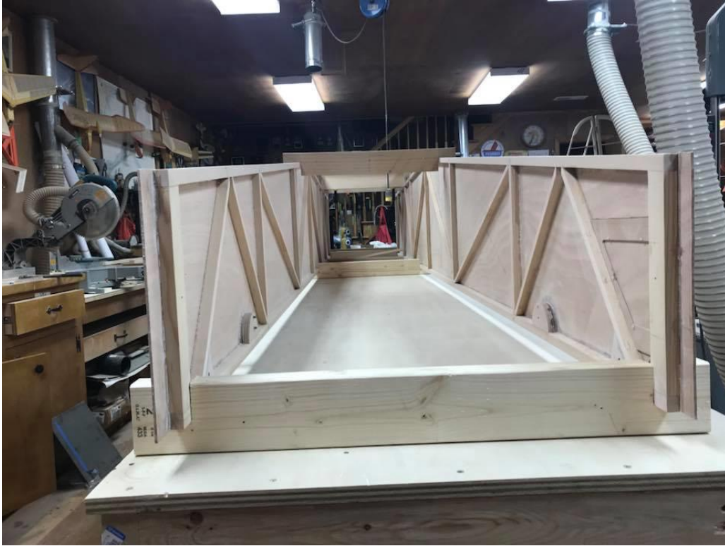
Figure 2: Fly Baby Fuselage Under Construction
