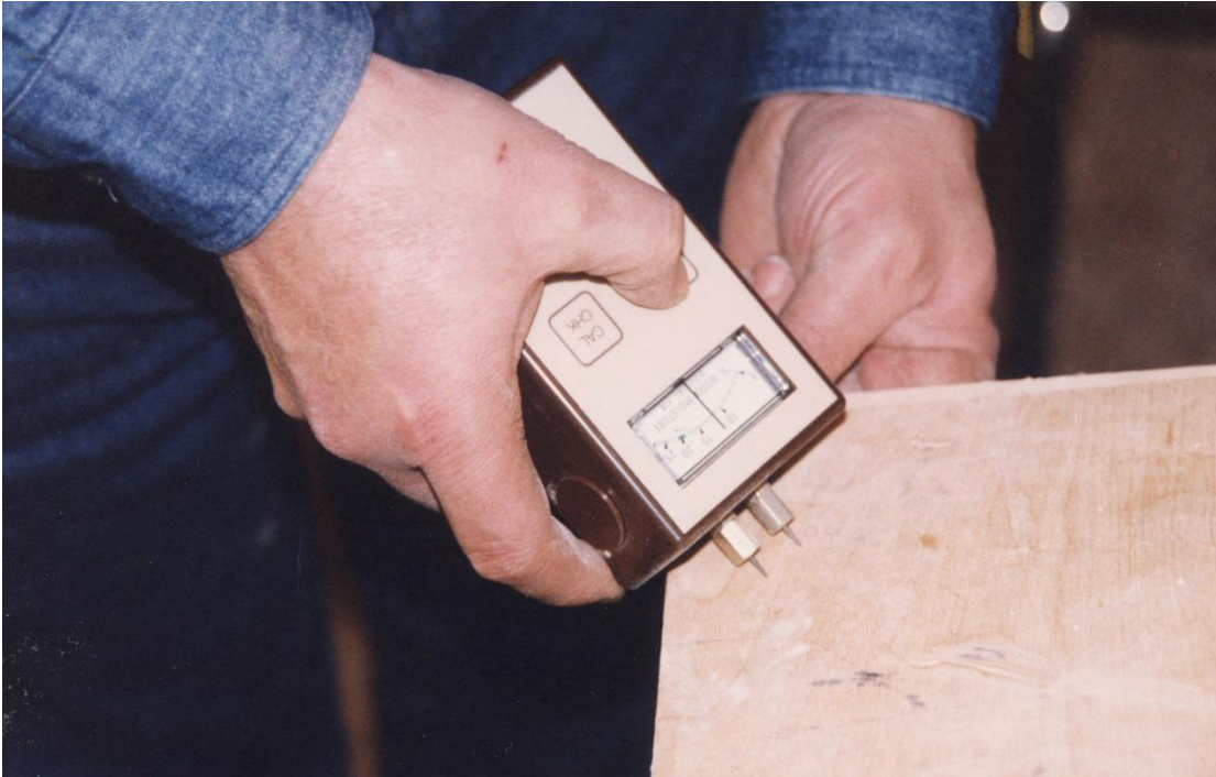
Figure 3: Measuring Wood Moisture
