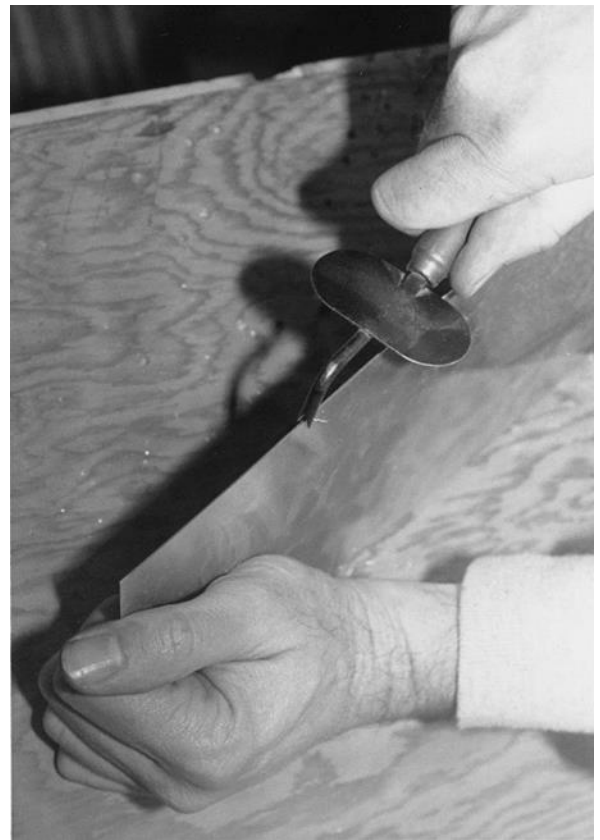
Figure 30: Edge Breaker in action
