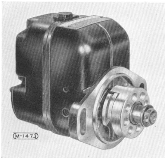
Fig. 1. Bendix-Scintilla Magneto Type S6RN-21, 3/4 Front View
