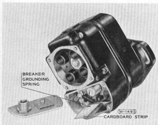
Figure 1. Paper Insulating Strip Under Breaker Grounding Spring
