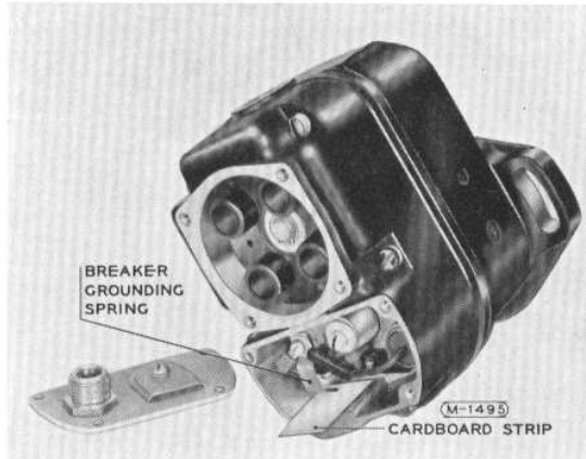
Fig. 27. Paper Insulating Strip Under Breaker Grounding Spring
