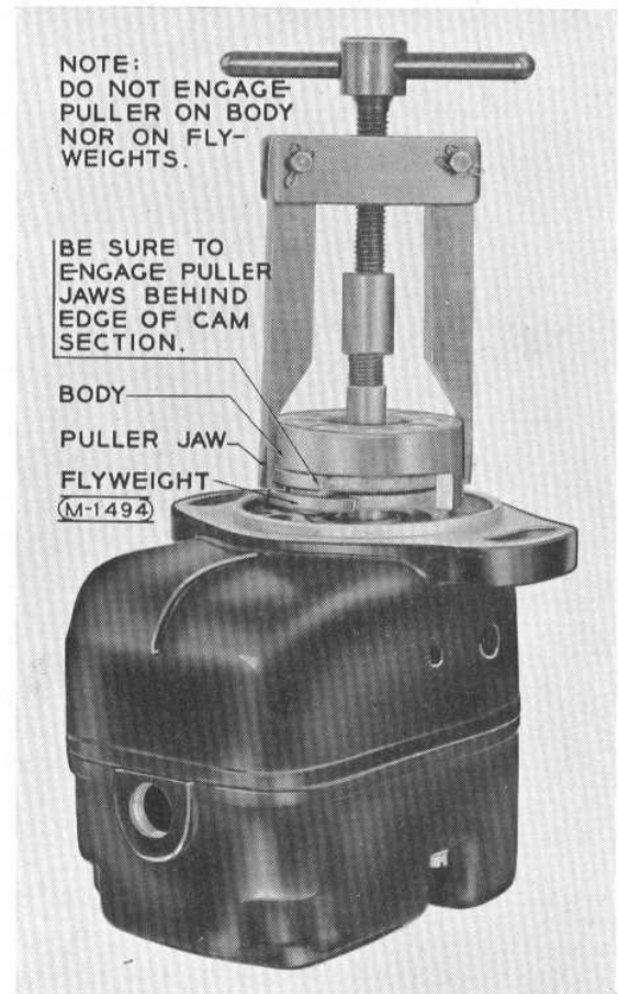
Fig. 25. Application of Puller to Impulse Coupling
