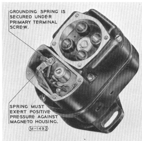
Fig. 24. Positioning of Safety Ground Spring on Breaker
