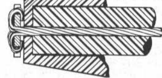
Fig. 13. Securing Strands to Washer
