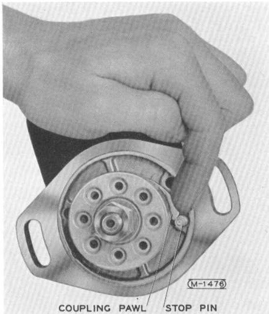
Fig. 4. Depressing the Impulse Coupling Pawls
