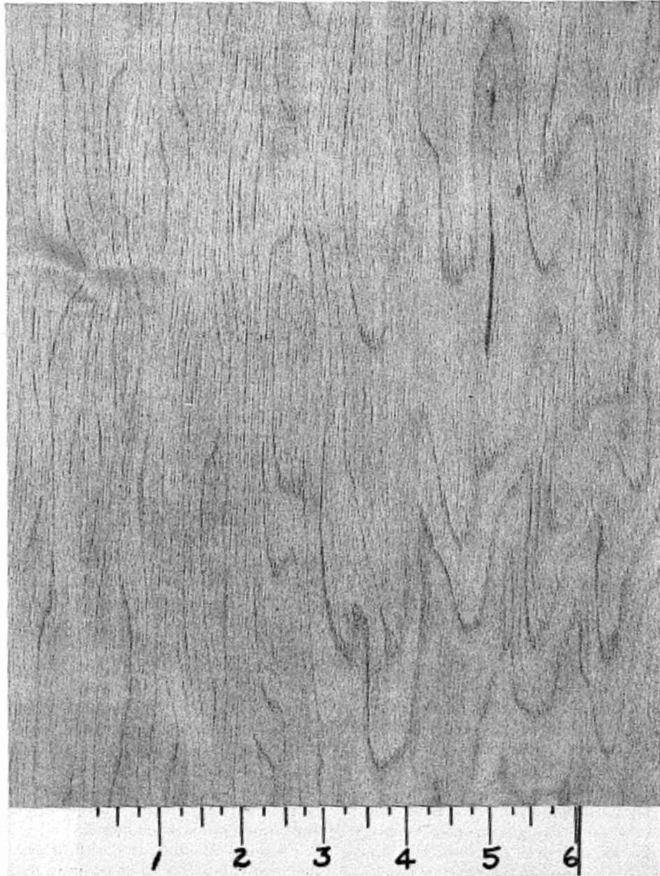
Figure 2-88. Objectionable rough cutting in maple.
