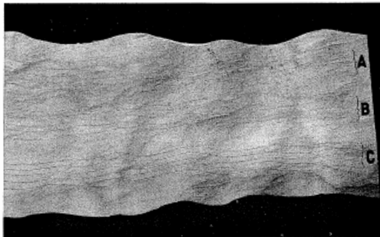
Figure 2-57. Tangential surface of wood tested with scribes to determine direction of grain. Note parallelism of scribe marks in same areas.
