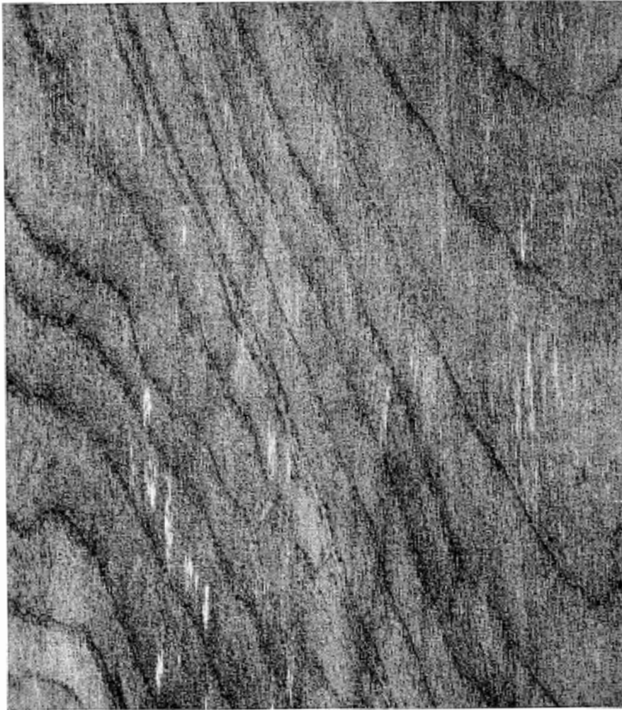
Figure 2-102. Fomes igniarius rot in rotary-cut yellow birch veneer.
