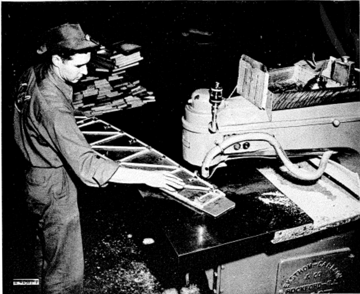
Figure 5-83. Routing wing ribs to contour.
