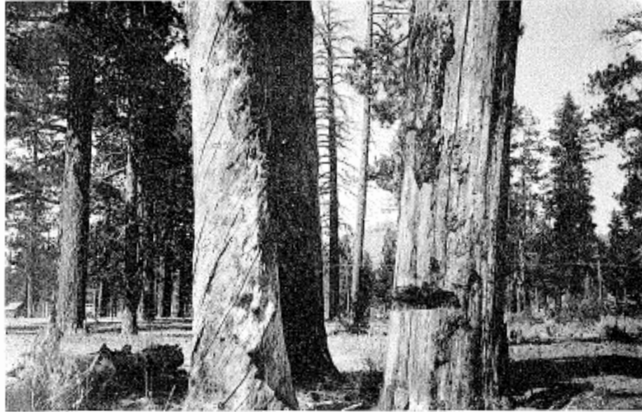
Figure 2-54. Straight grain and right-hand spiral indicated by direction of seasoning checks in dead tree trunks.
