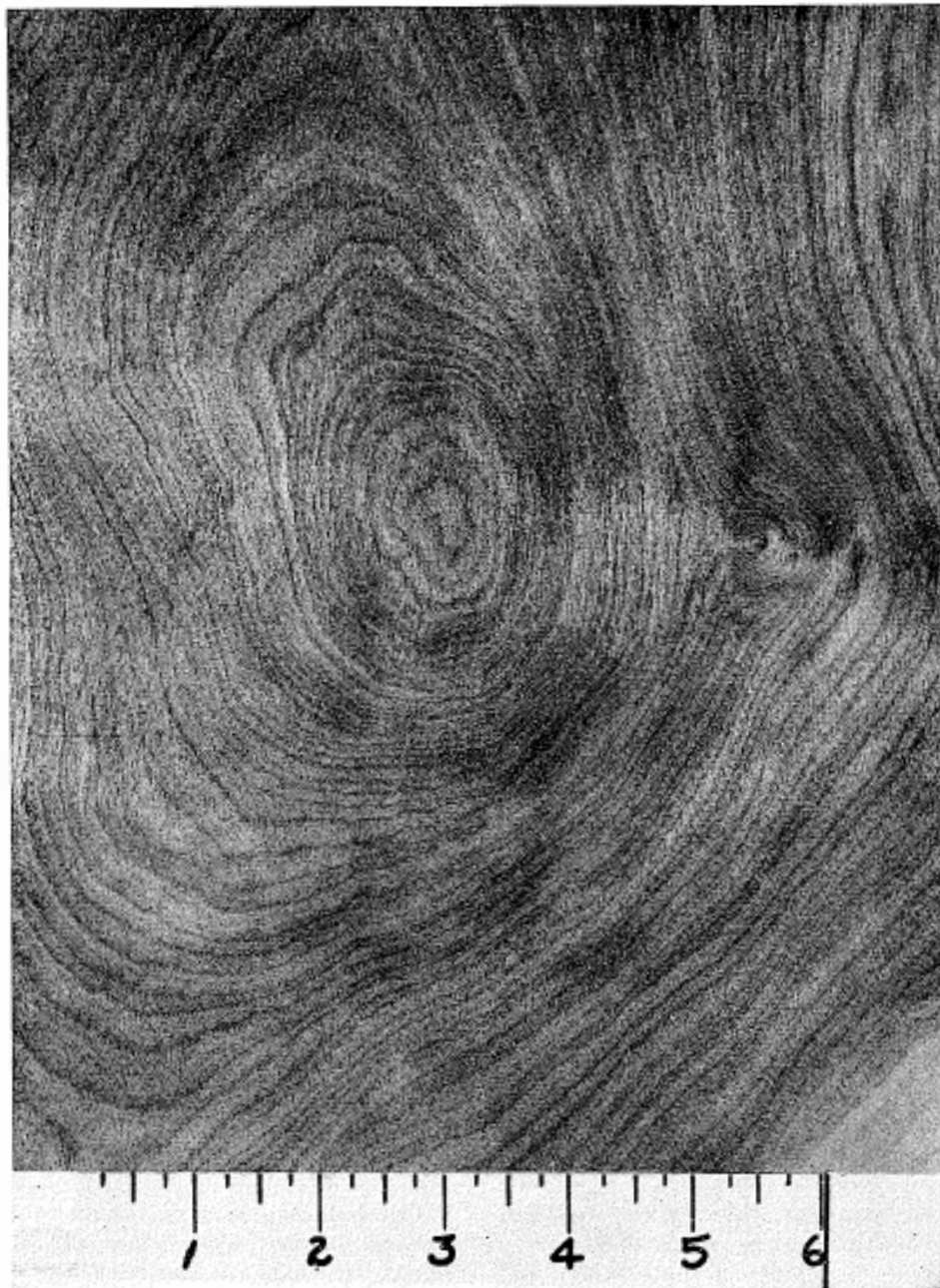
Figure 2-91. Cross grain resulting from small and large bumps.
