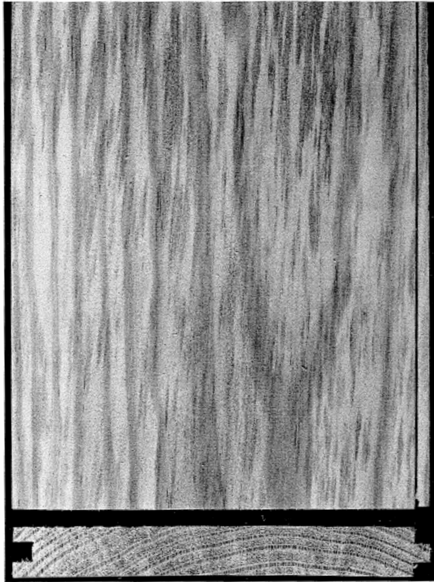
Figure 2-99. Planed southern yellow pine board showing typical sap stain.
