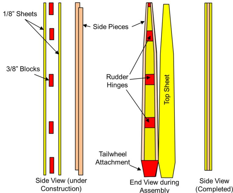
Figure 9: Rudder Post Construction
