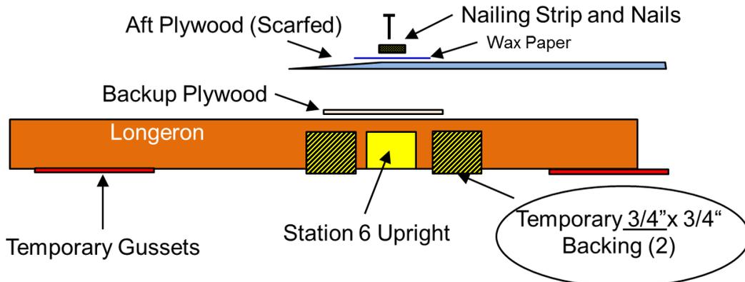
Figure 27: Station 6 Temporary Backing on the Right Side Truss
