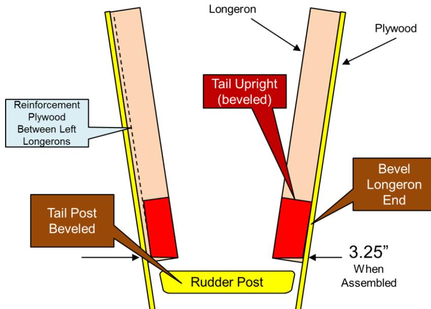
Figure 60: Beveling Needed at End of Tail
