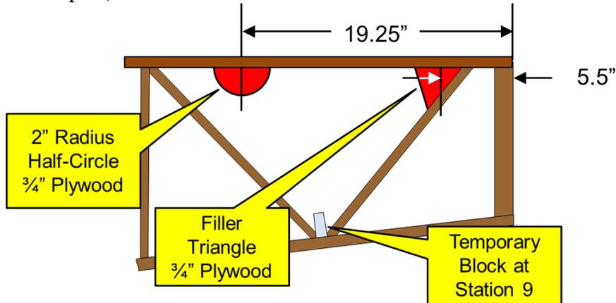
Figure 19: Horizontal Stabilizer Attach Points
