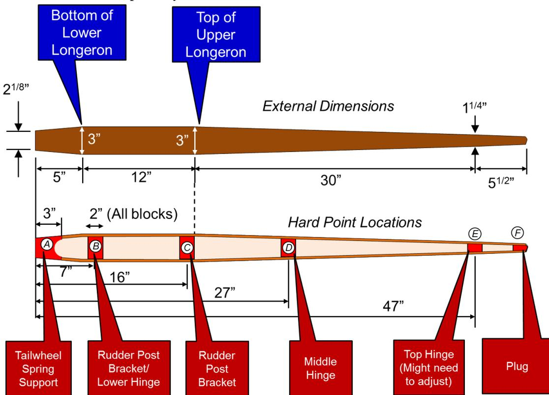
Figure 52: Rudder Post Dimensions and Uses
