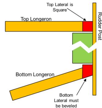
Figure 65: Bevel in Lower Lateral
