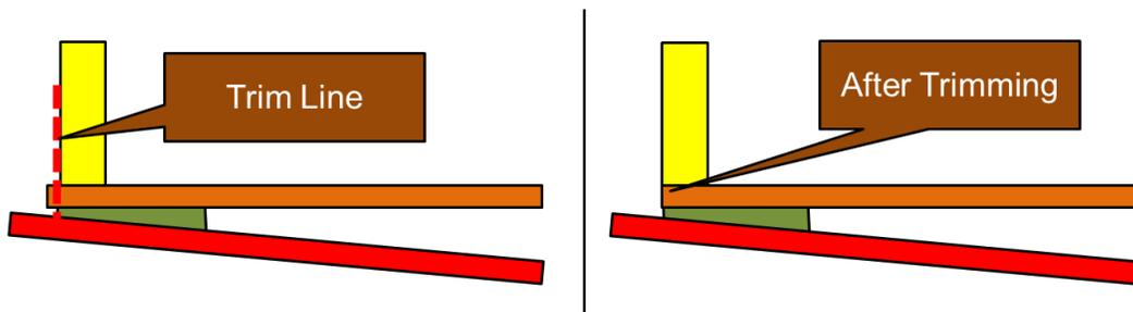
Figure 20: Trimming Above the Lower Longeron
