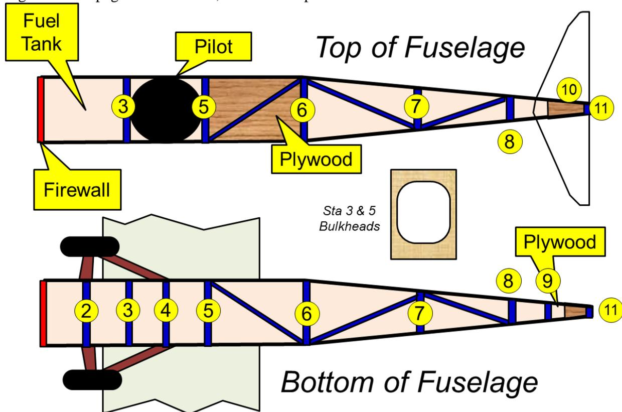
Figure 4: Top and Bottom Diagonal Bracing
