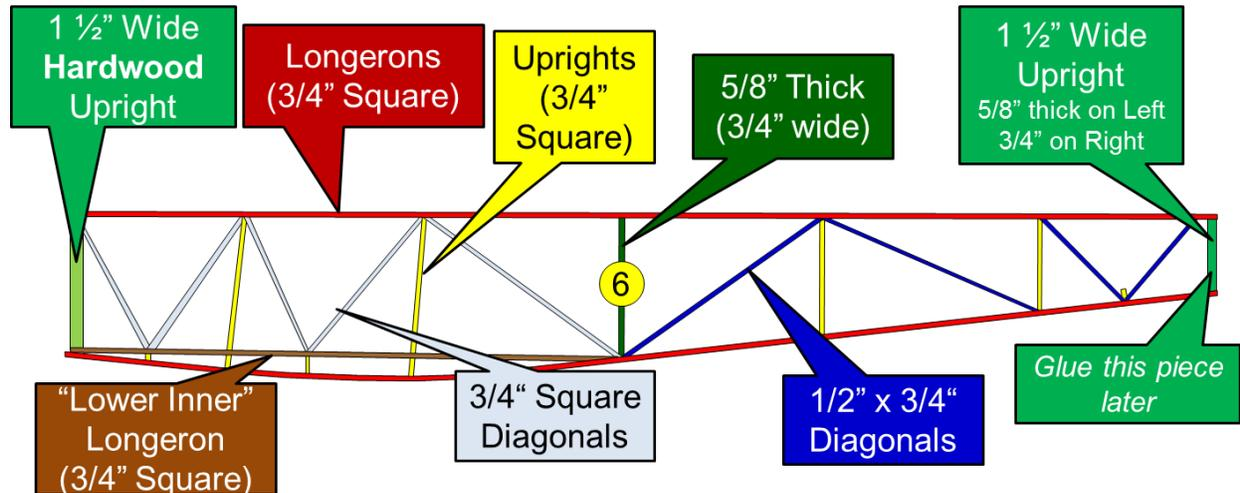
Figure 10: Fuselage Components
