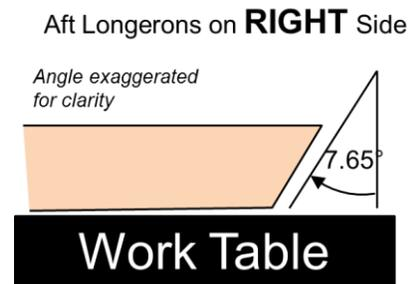
Figure 25: Aft Longeron Beveling on Right Side of Fuselage
