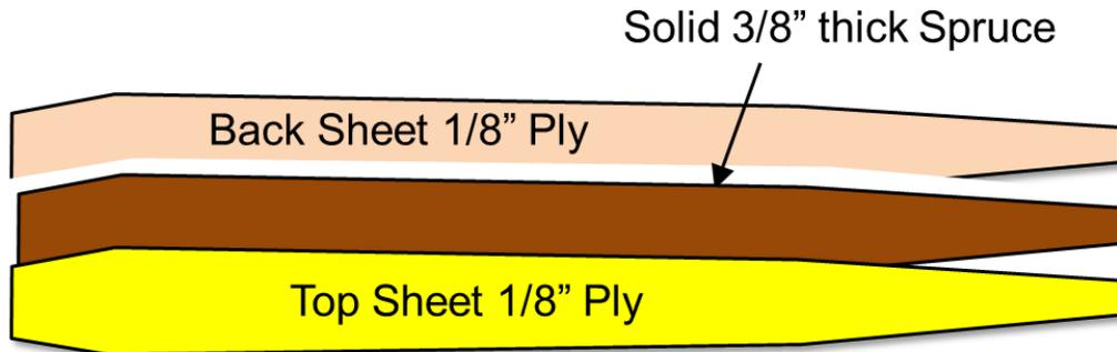
*Figure 56: Solid-Core Rudder Post*
