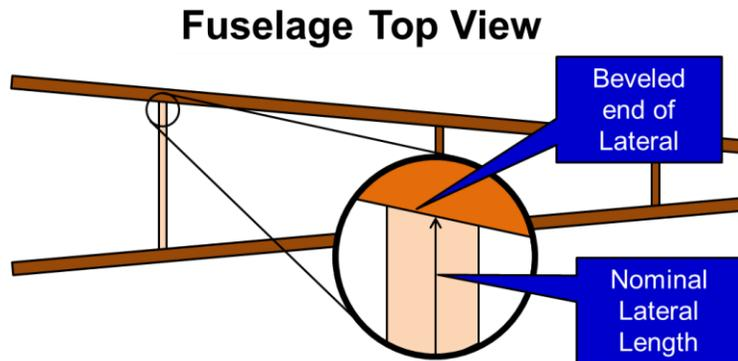
Figure 44: Beveled Ends of Lateral Braces
