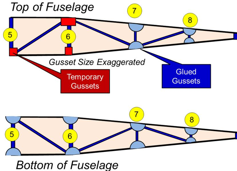
Figure 49: Gusseting the Aft Fuselage
