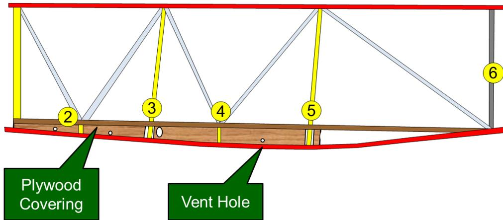
Figure 43: Lower Fuselage Box Structure
