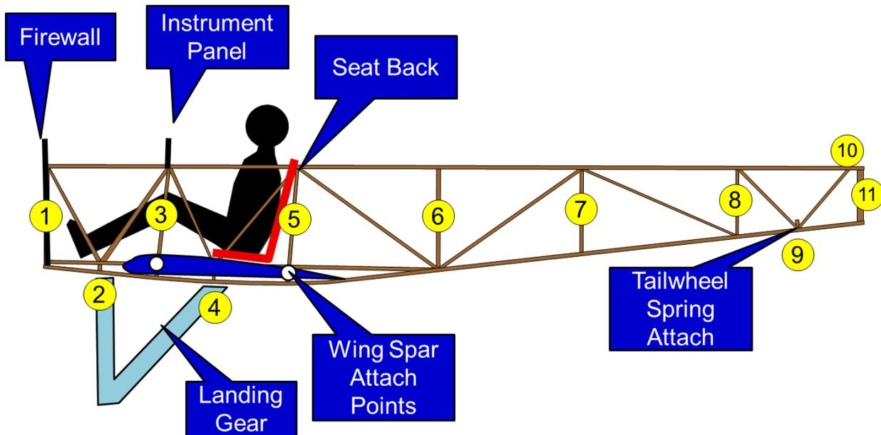
Figure 3: Fuselage Stations
