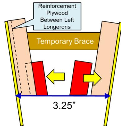
Figure 59: Setting the Tail Spacing
