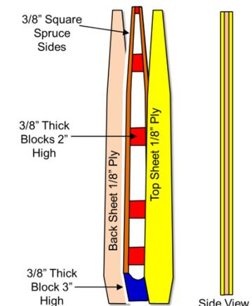
Figure 51: Stock Rudder Post Construction
