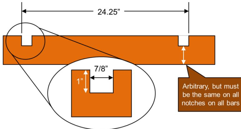
Figure 31: Fuselage Spacer Bars
