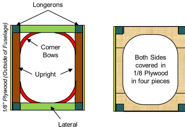
Figure 29: Bulkhead Construction
