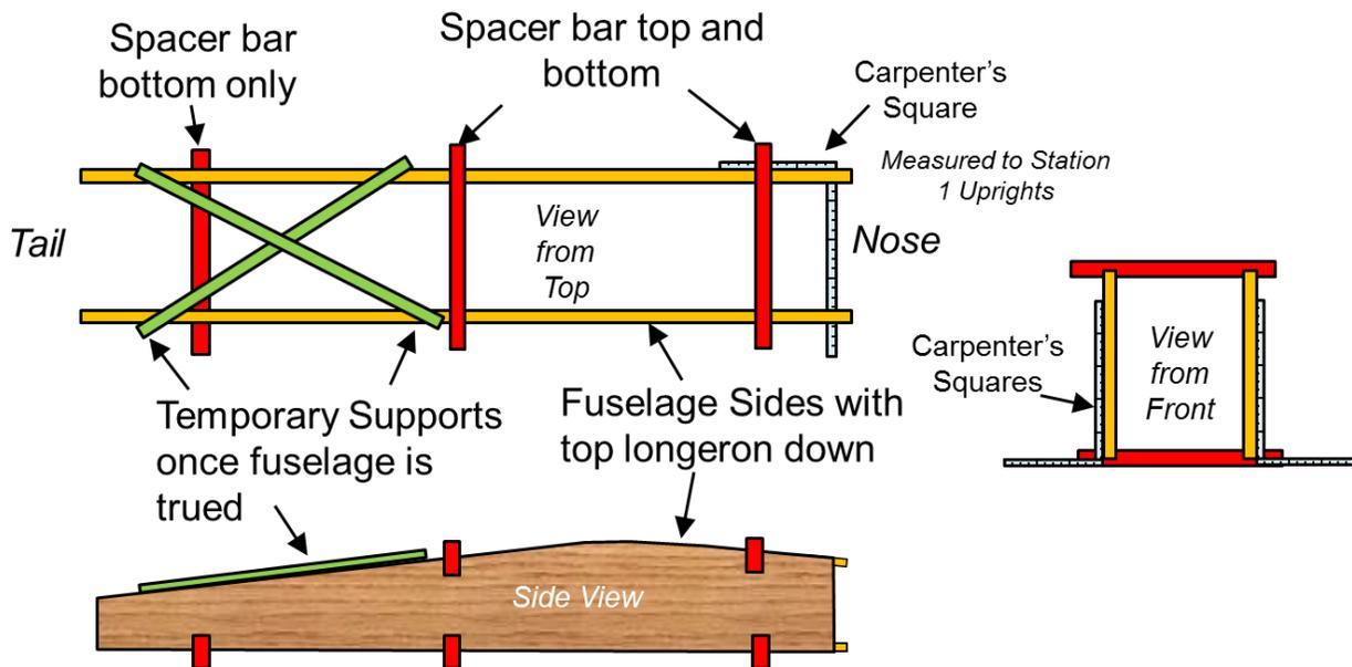
Figure 32: Aligning the Fuselage Sides
