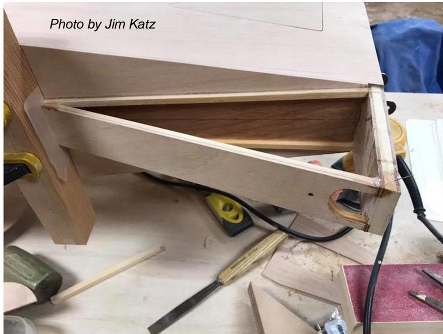
*Figure 69: Tail Skeg Under Construction*
