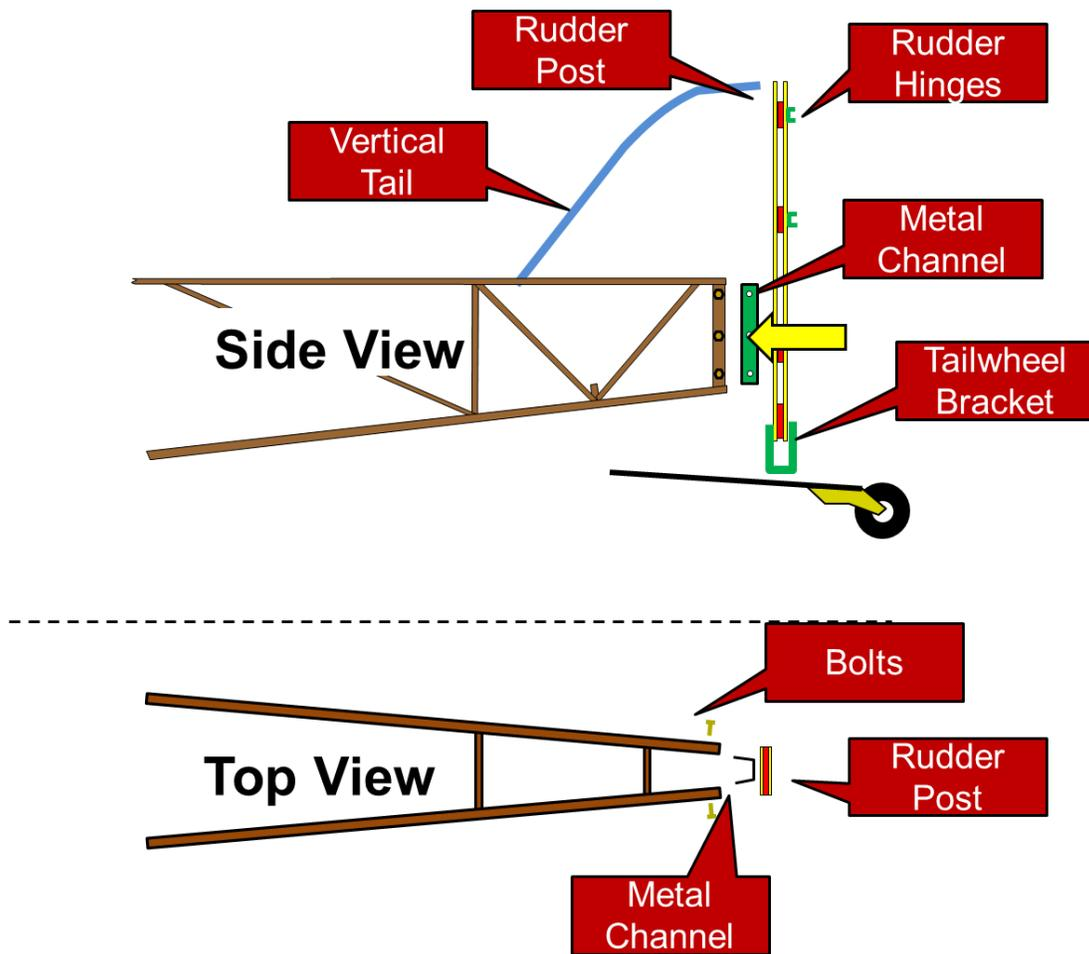
Figure 50: Rear Fuselage Joining
