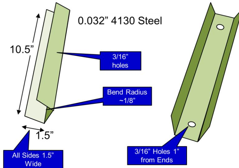
Figure 57: Rudder Post Bracket
