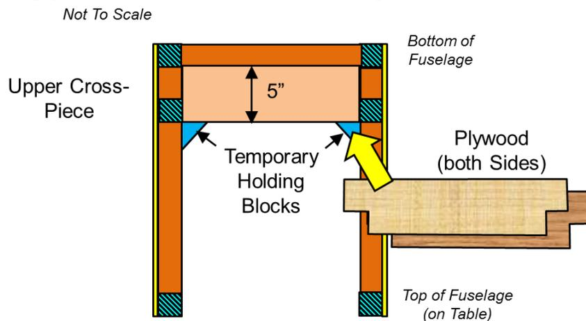
Figure 41: Station 4 Construction
