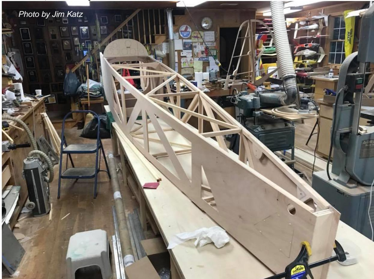
*Figure 1: Fly Baby Fuselage Under Construction*
