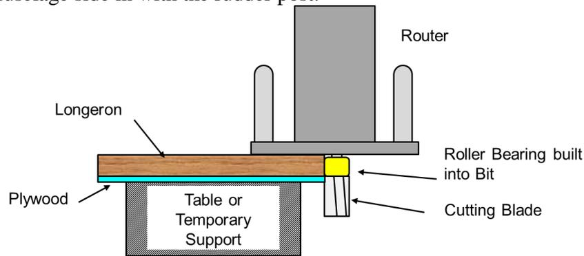
Figure 23: Trimming Plywood with a Router
