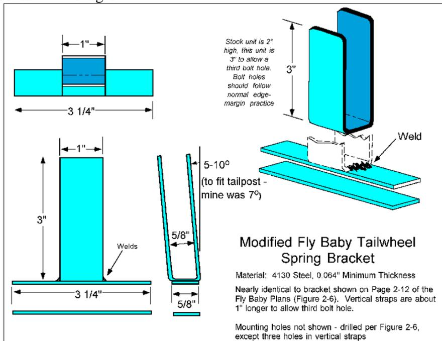
Figure 55: Modified Tailwheel Spring Bracket
