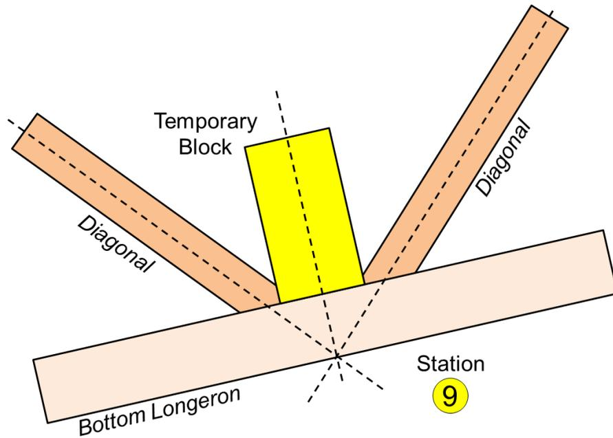
Figure 18: Station 9 Diagonal Positioning
