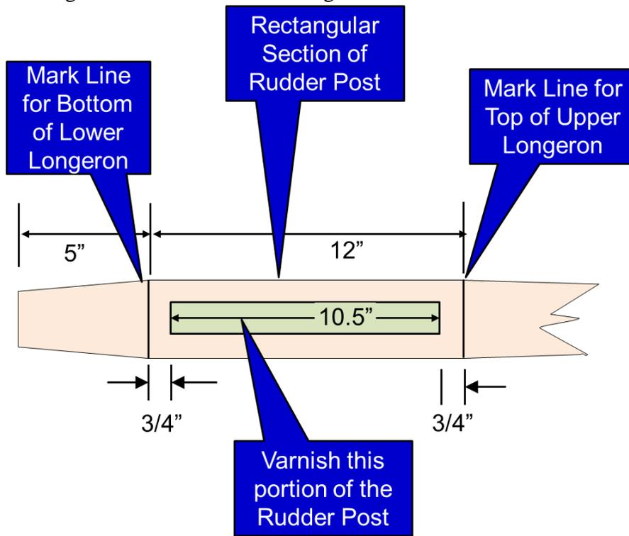
Figure 58: Rudder Post Preparation
