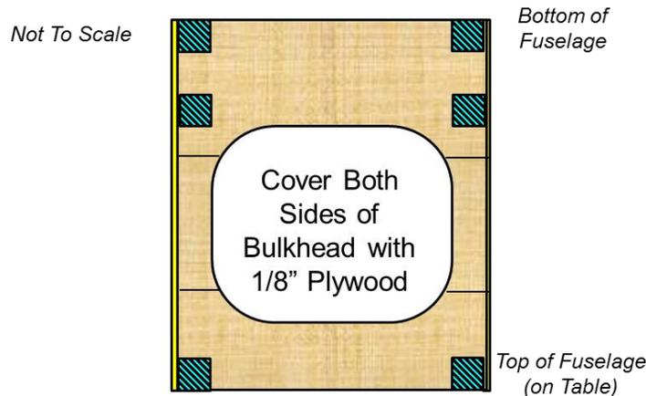
Figure 37: Completing the Bulkhead
