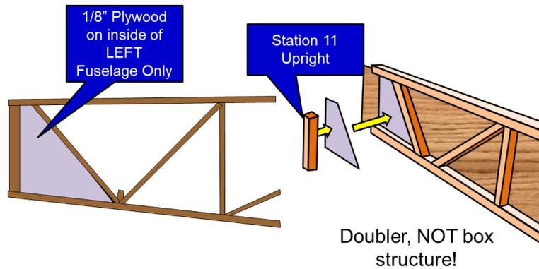
Figure 62: Aft Fuselage Doubler (Left Side Only)
