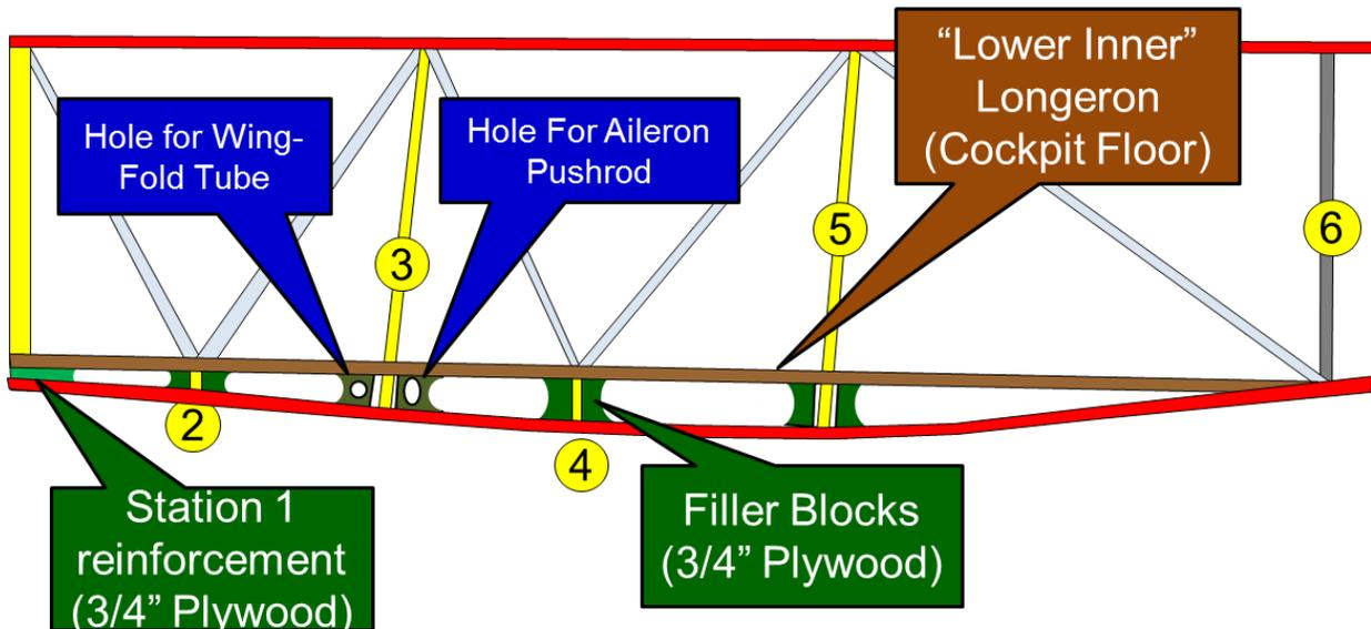
Figure 42: Lower Longeron Reinforcement
