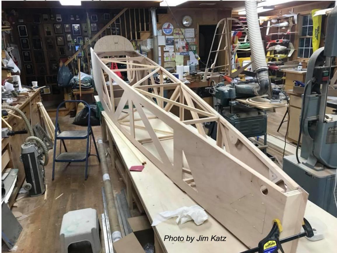
*Figure 71: Routed Fuselage*
