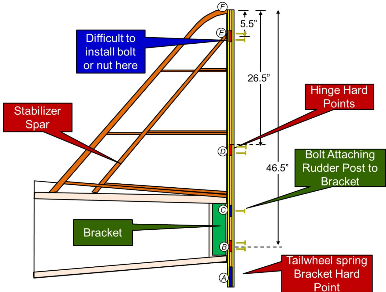
*Figure 53: Interference Issue with Upper Hinge Point*
