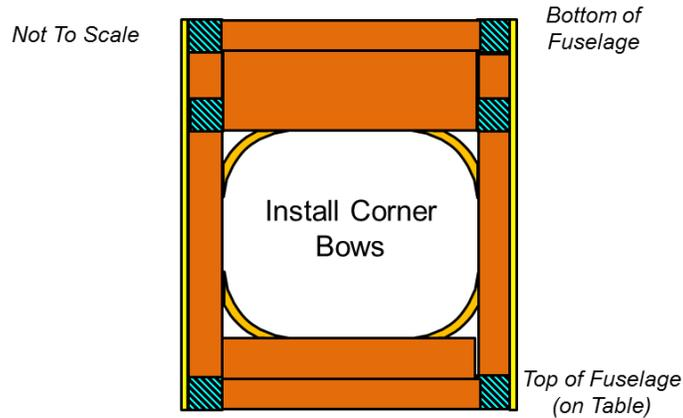
Figure 35: Install Bulkhead Arcs
