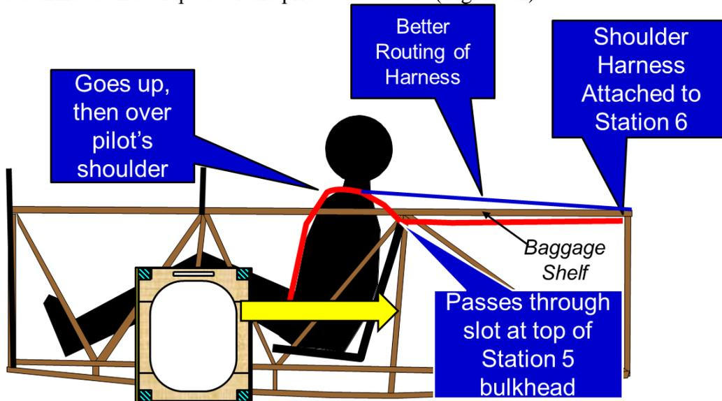
Figure 72: Shoulder Harness Routing
