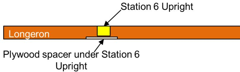
Figure 24: 1/8" thick spacer under the Station 6 Upright
