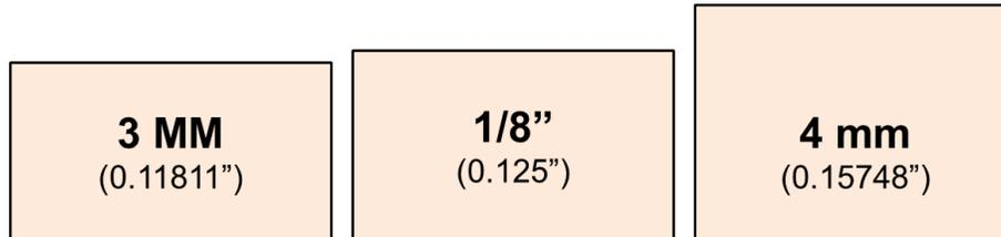
Figure 8: *Relative Thicknesses of Metric Plywood vs. 1/8 inch Plywood*
