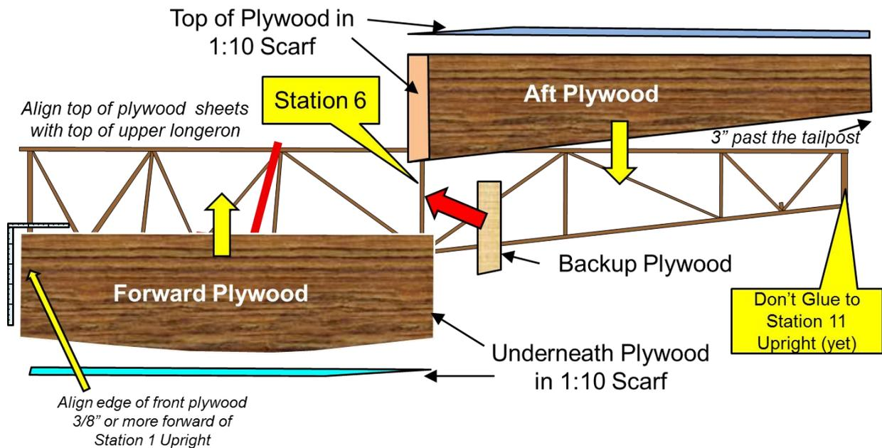
Figure 21: Fuselage Plywood
