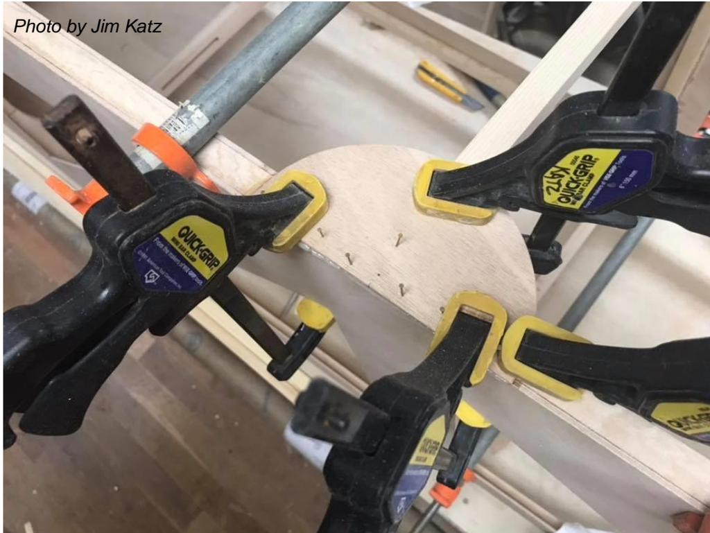
Figure 47: Gluing the Gussets
