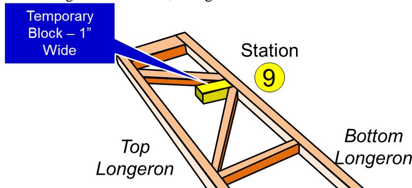
*Figure 17: Temporary Block at Station 9*
