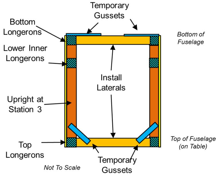
Figure 33: Installing Laterals at Station 3
