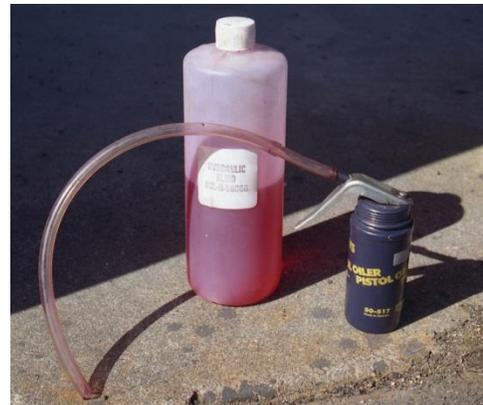
Figure 21: *Oil Can Brake-Fluid Pump*
