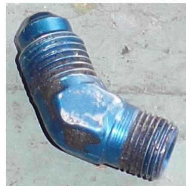
Figure 20: AN Flare and Pipe Thread
