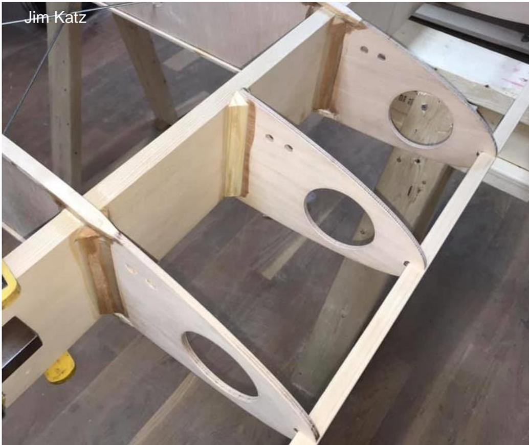
*Figure 33: Holes in Nose Ribs for Pitot/Static Plumbing*
