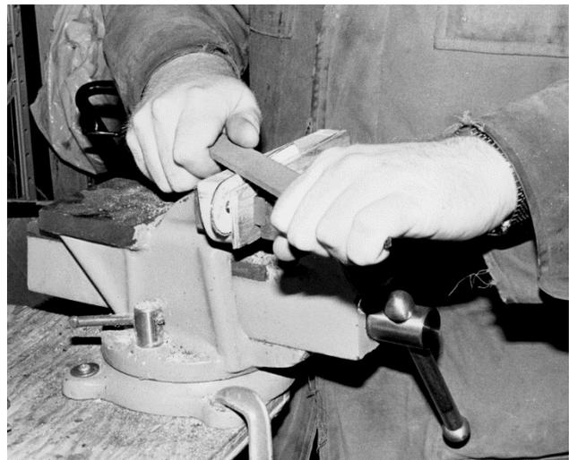
The cut describes whether the file's teeth are long and parallel or small and diamond-shaped: single cut and double cut, respectively; the double cut is more effective at removing metal.
