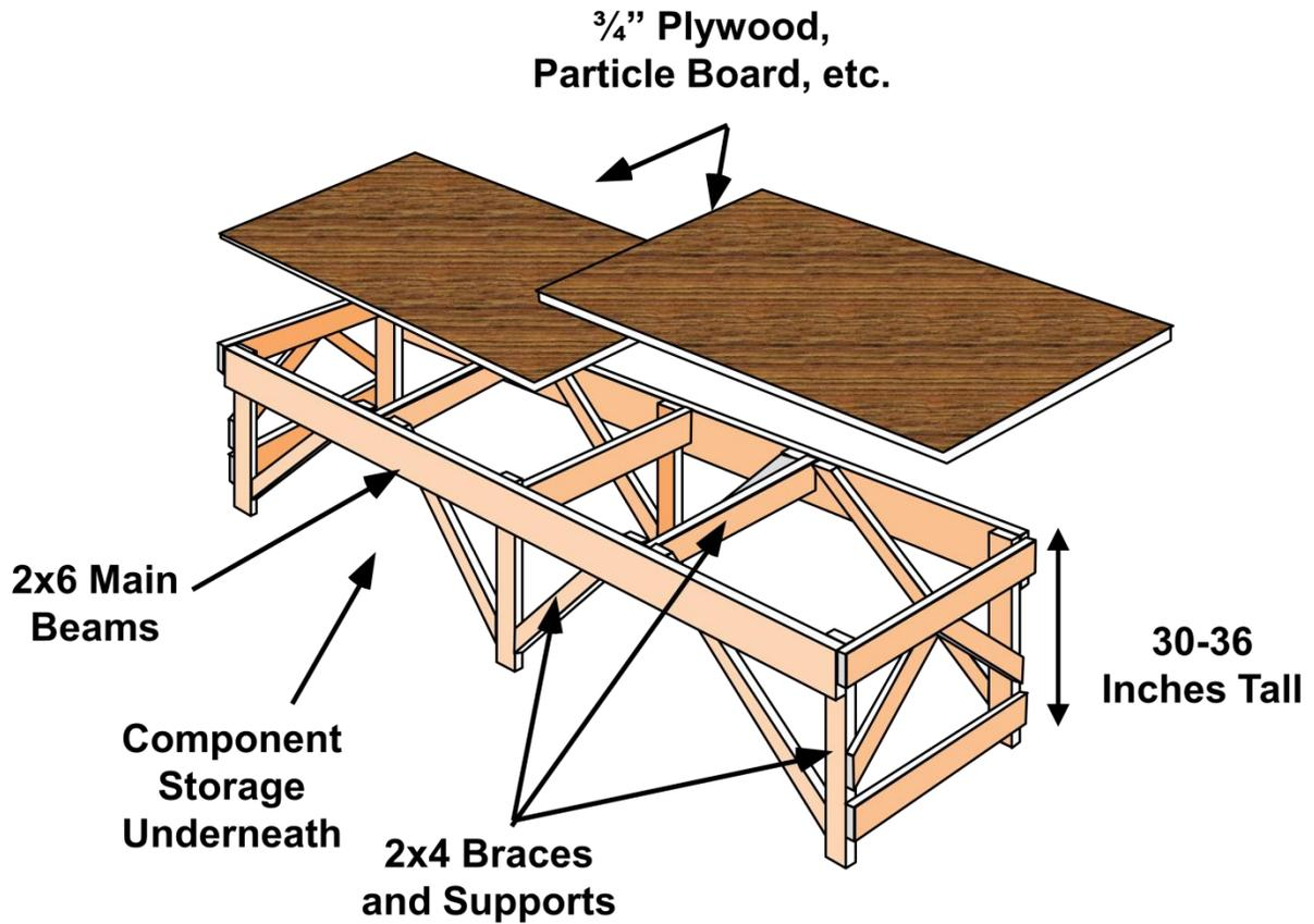
When you can, use screws instead of nails...nails tend to loosen over time, and screws are easier to remove if you decide to scrap the table at the end of the project.
