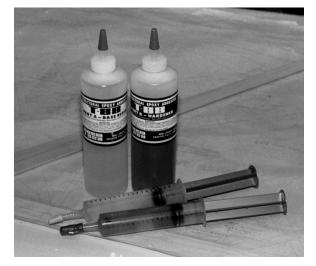
They're a bit more expensive, not really a drawback, these days. However, they should not be used in low temperature conditions. Their ultimate strength depends on the temperature when they cured. So if you're working in the cold climes in a garage, might want to add some heat.
