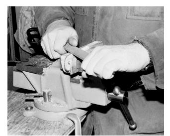
The <u>cut</u> describes whether the file's teeth are long and parallel or small and diamondshaped: <u>single cut</u> and <u>double cut</u>, respectively; the double cut is more effective at removing metal.
