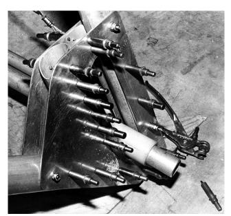
that point on, each additional hole will maintain proper alignment.
