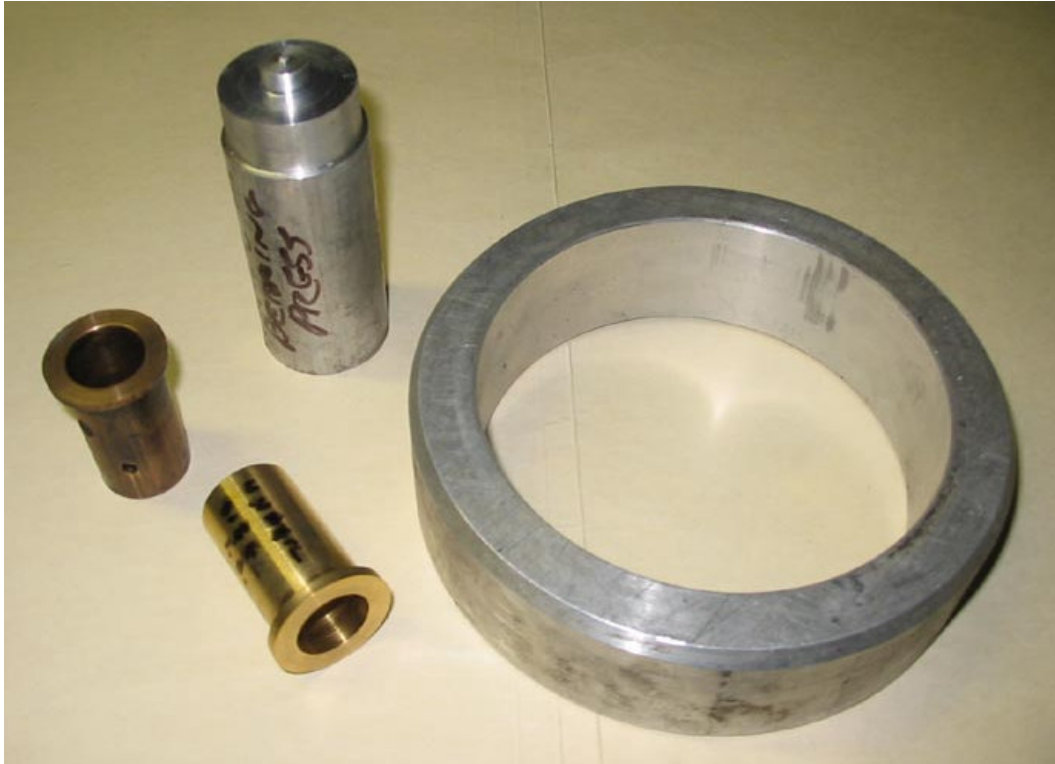
Figure 9: Clockwise from top left: homebuilt wheel bearing press; homebuilt ring for breaking pneumatic tyre's bead from rim; homebuilt brass bushing; and old Iolite bushing, note holes for grease nipple and anti-shimmy device.
