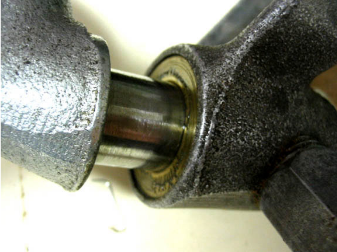
Figure 3: Fork to Oilite Bushing bearing area.
