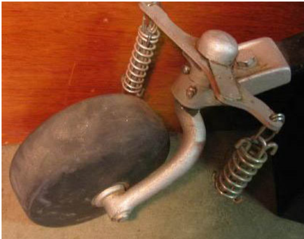
Figure 1: Maule model SFSA "solid" tailwheel. Note dissimilar safety springs and absence of anti-shimmy damper.
