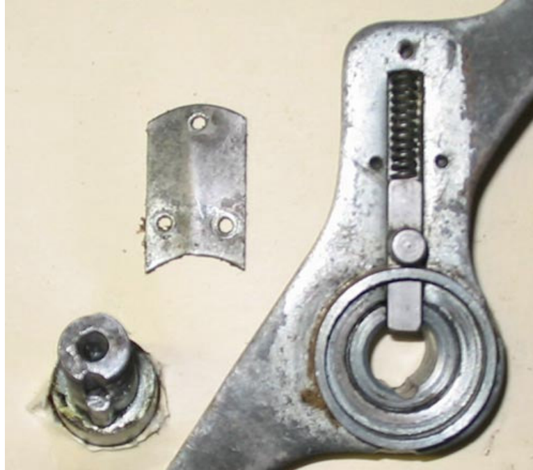
Figure 6: Assembled Steering Arm Assembly [6], displayed bottom side up for clarity, along with the top portion of the Fork [26]. Note the Lock-Ring Pin on the Fork and corresponding detent/keyway in the Lock Ring [4] itself .
