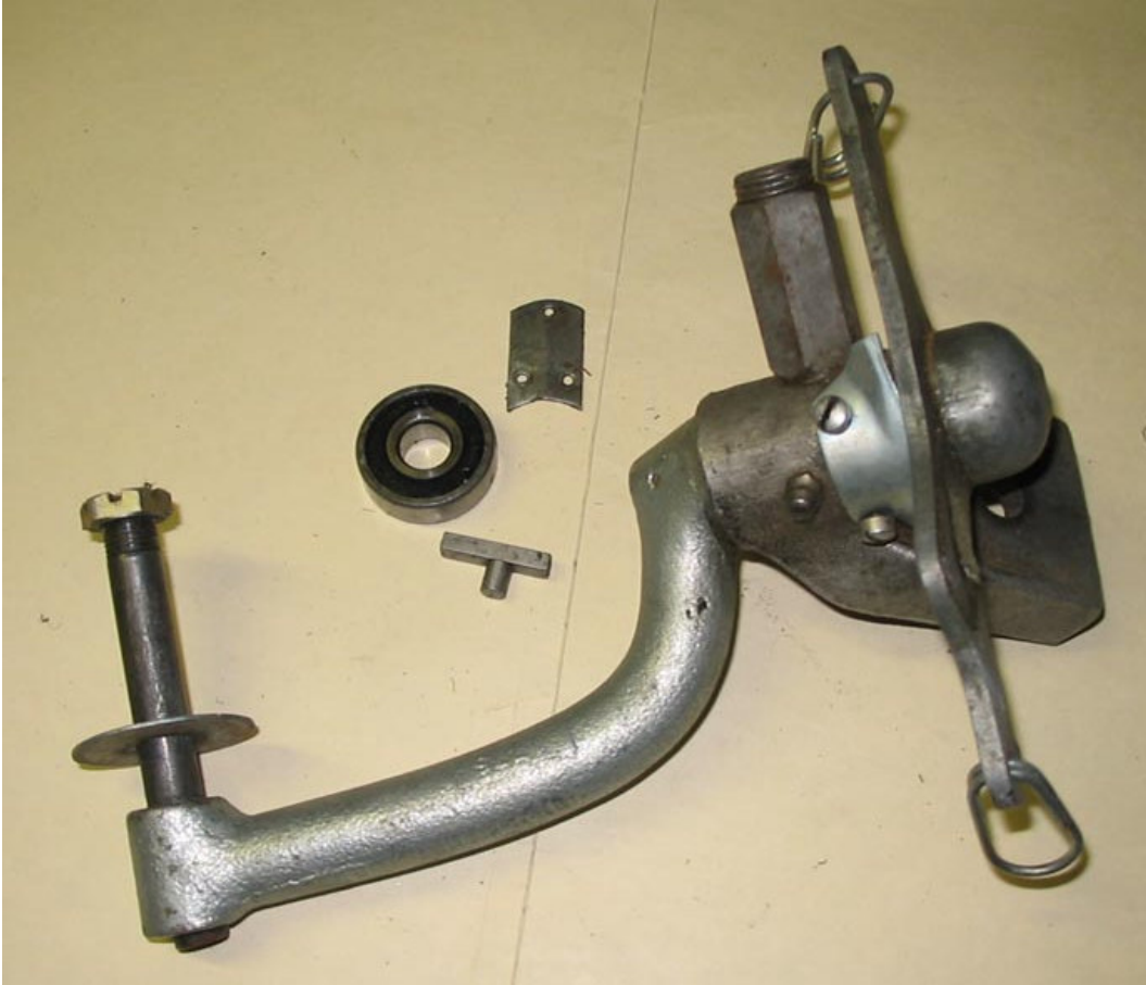
Figure 10: partially assembled tailwheel
