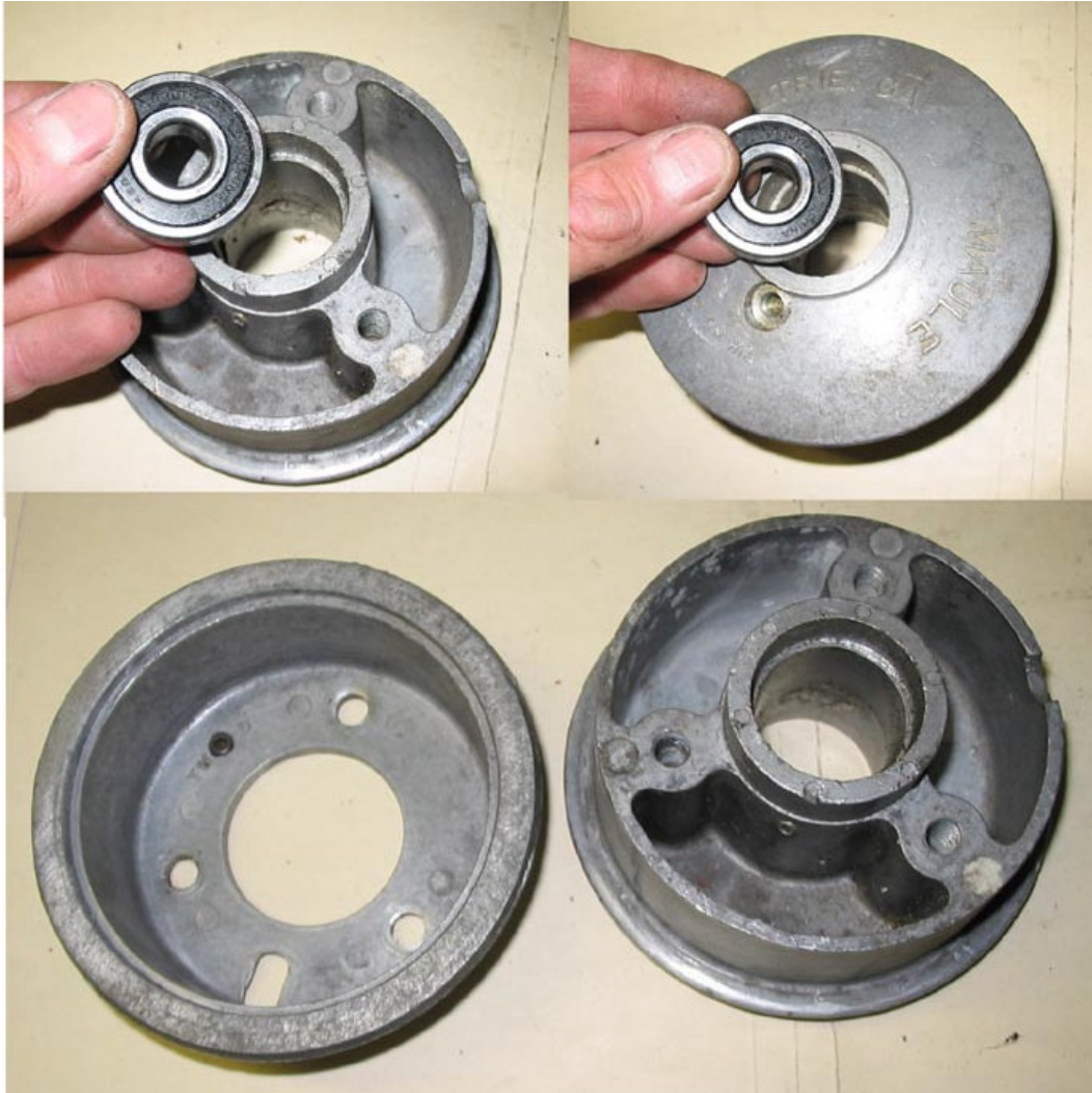
Figure 8 (collage): SFS-P8A "pneumatic" wheel components. Note that the non-bearing wheel half has damaged hub-cup circlip-ring groove, which has been cleaned up on a lathe. A STANDARD Maule hubcap, or perhaps a cut-to-fit piece of aluminum or plastic sheet could be siliconed in place for an inexpensive repair?
