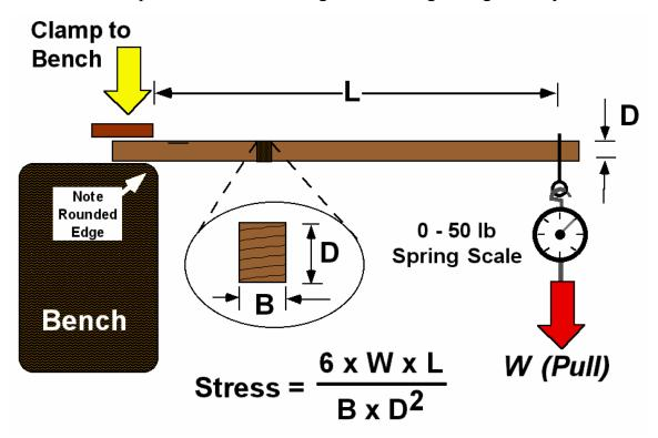
I test at least one sample from each board to destruction to find its strength, using the same 0 to 50 lbs dial spring scale. They cost about \$15, nothing fancy.
